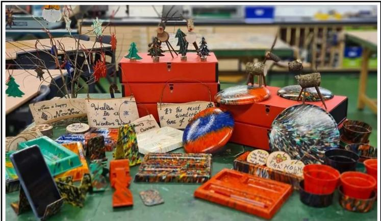
Plastic from shredded waste, generated by the bird feeder DT project, along with other plastic collected from around school, has been made into sheets and then vacuum formed into Frisbees, desk tidies and pots; or cut and bent into shapes to make phone holders and
